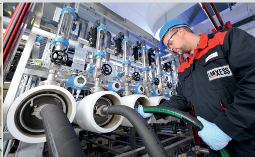
For quality assurance purposes each individual Lewabrane® element is checked in an element tester.
